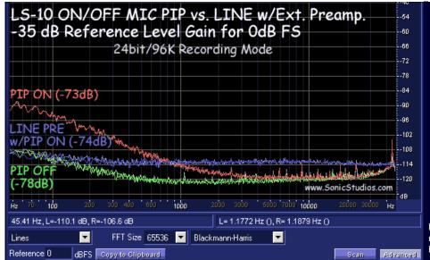
knob set at #9 was used, while the LINE input was measured adjusted to #8 with external <u>PA-3SX</u> at highest #3 gain.
