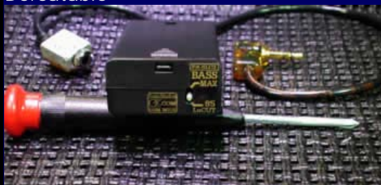
PA-6LC2 .... 85 Cycle Bass Filter .... Switch Defeatable
